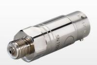
PCM161 pressure sensor allows a combined pressure and temperature measurements at a same location. Wetted parts being all stainless steel, it is compatible with all common and hostile pressure media used in aerospace and automotive. Miniature dimensions, low mass and ruggedized design make PCM161 pressure sensor well adapted to embedded applications on vehicules, aircrafts, missiles, satellites, etc.
