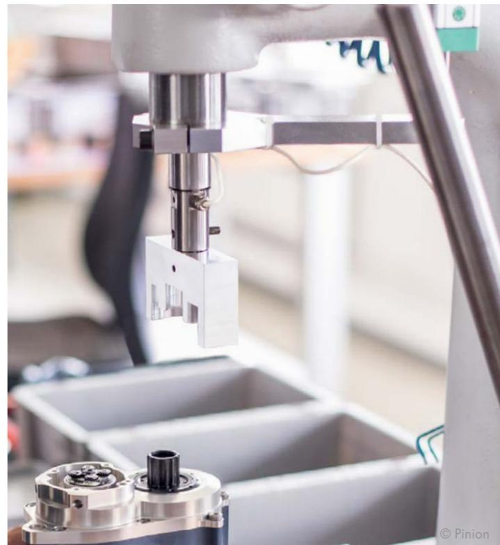
The standard setup is to fit the load cell as an extension of the press ram, so that it measures the applied force directly inside the axis (directly at the tool). The displacement transducer (optional) moves co-jointly with the travel of the press ram, travelling in parallel with the ram axis at the side of the press head.
