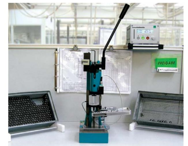
Our **how-to-do video** shows how to fit the load cell and displacement transducer to a manual press. It is available to download from: <http://goo.gl/MBkWMN>
