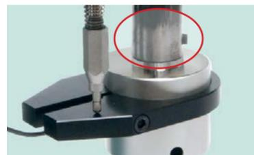
Ram with internal bore and grub screw
