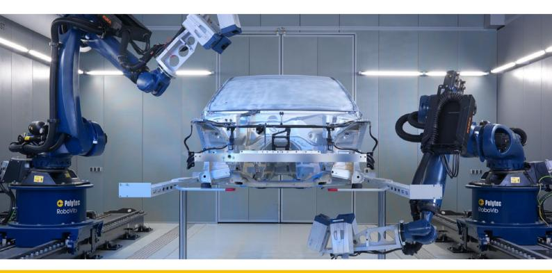
**RoboVib® Structural Test Station** Automated Experimental Modal Testing Product Brochure
