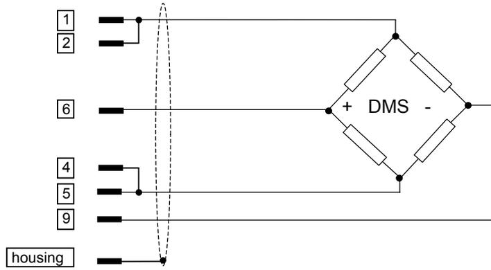
**Connect strain gage sensors with sense line**
