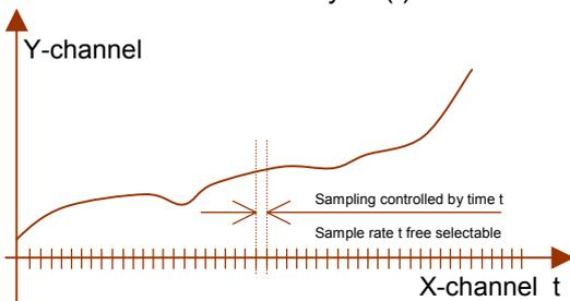
A measurement value on channel Y is logged as a function of time t.
