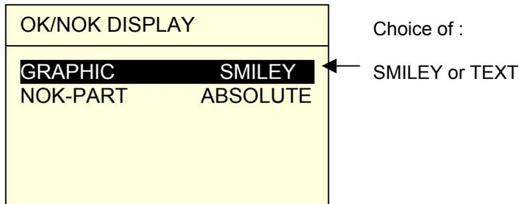
By using the < ↓ > -key go to line GRAPHIC. With the < ⇒ > -key you select the display form:
