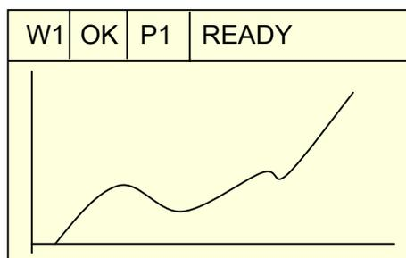
If you configure the DIGIFORCE® for the first time you will not see a measurement curve, yet. For the scaling of the axis there is no reference point defined. As a result we recommend to switch on the function AUTOSCALE at first:
