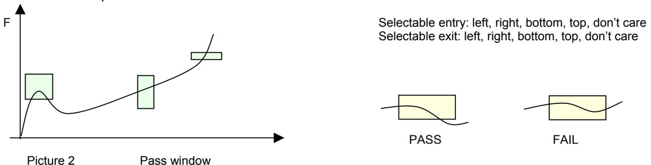
**Important!** The Measurement Curve must not start in the X-range of the PASS window! Otherwise the DIGIFORCE sends out a NOK-signal although the respective window might have been passed the correct way:
