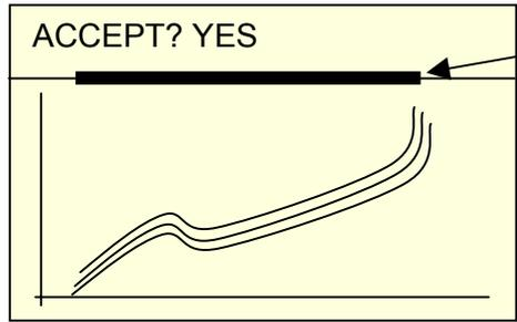
Starting with the second curve, an additional bar will appear in the graphic. It stands for the "band width" of the present measurement curve. This helps to avoid acceptance of curves that are too short as this is difficult to differentiate in the graphic alone.
