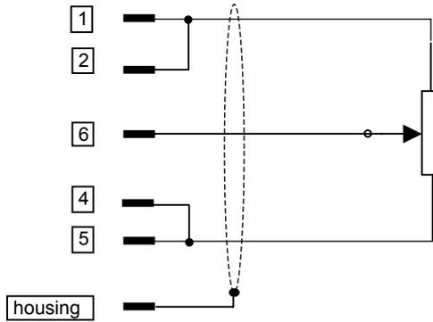
**Connect sensors with standard signal**
