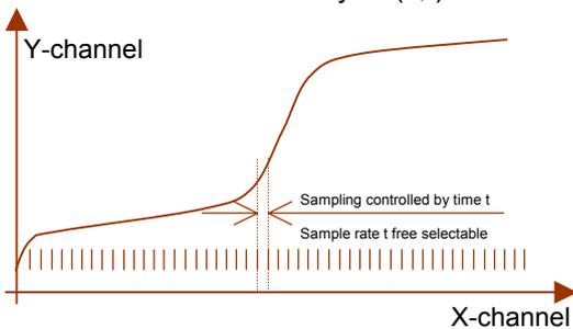
One measurement value Y is saved as a function of measurement value X. A selectable time rate determines the reading of the X-Y-value pairs.
