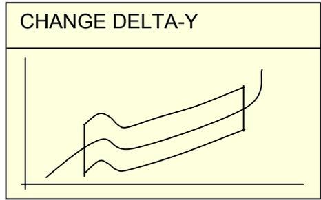
Press again the < ↵ >-key! Now you can correct the envelope curve limits numerically which you just created graphically. Moreover, the envelope curve can be switched ON/OFF and the trend-tracking can be activated.
