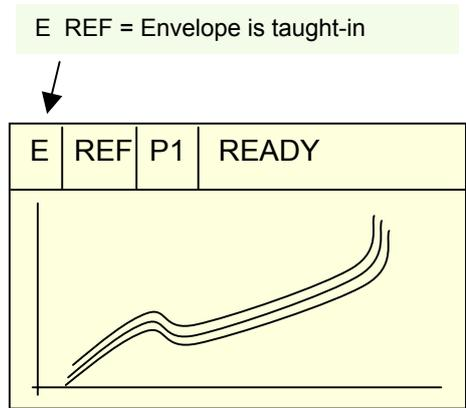
Similar to the window editing routine you are lead through the envelope configuration path by pressing < ↓ > repeatedly. First of all, the beginning of the envelope curve (X-MIN) is set. In order to do so, a dotted vertical line appears on the left side of the display. This can be moved with the ← → -keys to the place fo the reference curve where the envelope curve control should start:
