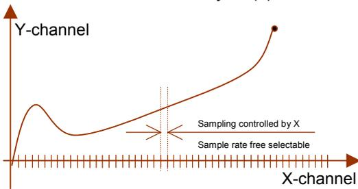
A Measurement value Y (force) is displayed and evaluated as a function of a measurement value X (displacement). A selectable X-sample rate defines the reading of the X-Y-value pairs.
