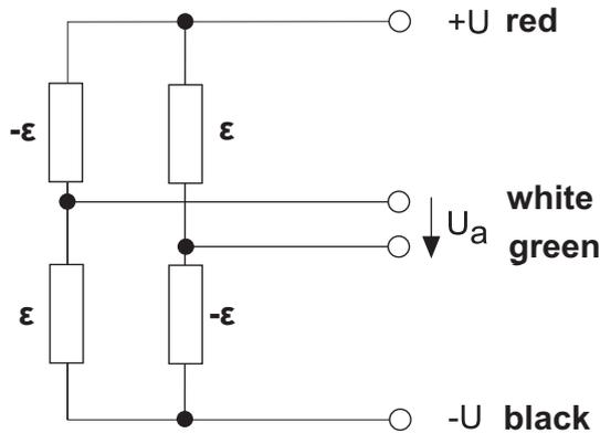
Figure 3: Full-bridge strain gage models 8413 and 8414
