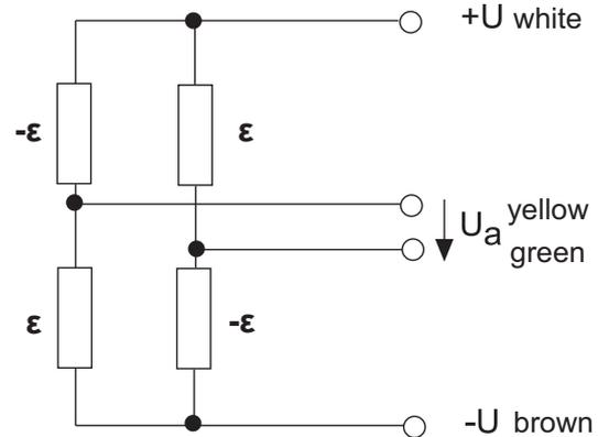
Figure 4: Full-bridge strain gage models 8415 and 8416
