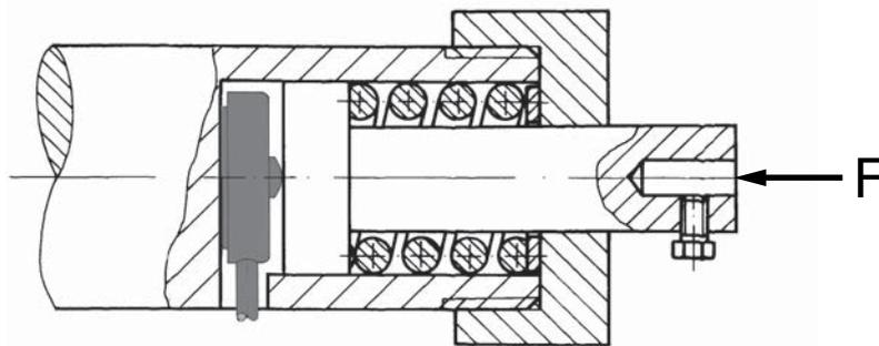
Figure 5: When using a spring element to mount the sensor, an initial load is applied to hold the sensor in position.
